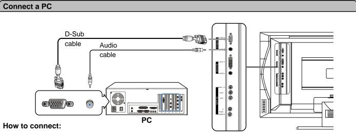
Connect a D-Sub cable between the S-Sub interface on the PC the D-Sub interface on the unit.
